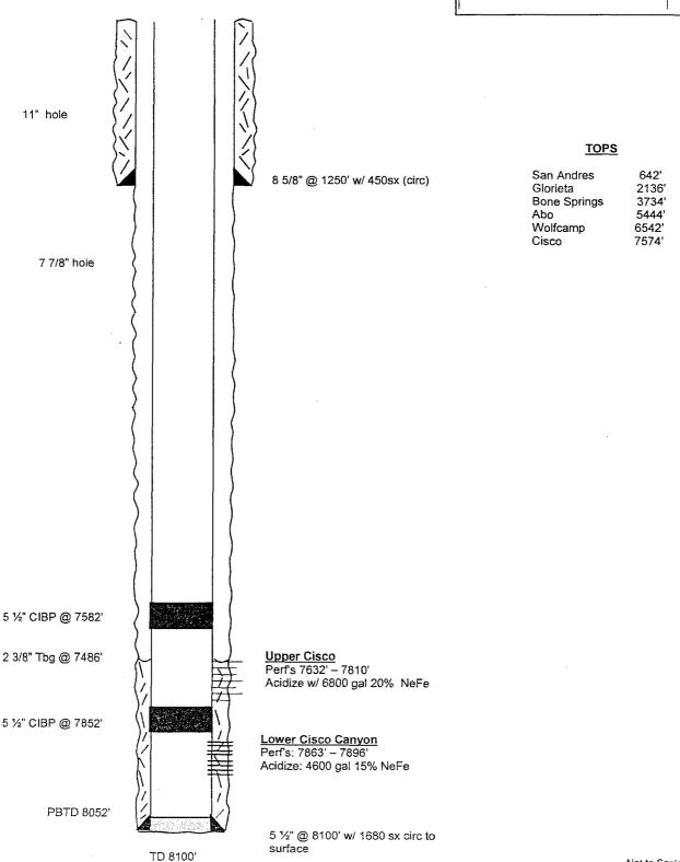
WELL NAME: Dagger Draw 30N Com #5 Field: Dagger Draw - Upper Penn LOCATION: Unit B, Sec 30, T19S-25E 990' FNL & 1980' FEL Eddy County, NM GL: 3555' ZERO: **KB**: 3571' 8 5/8" 32# K-55 1250' **SPUD DATE**: 11/19/87 **COMPLETION DATE**: 1/24/88 5 1/2" 17# J-55 ST&C 8100' COMMENTS: **BEFORE** TA
