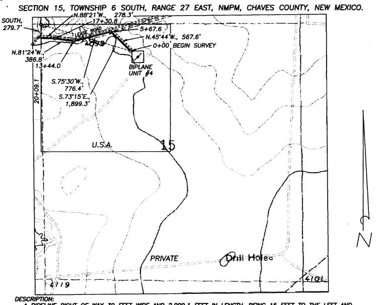
A PIPELINE RIGHT OF WAY 30 FEET WIDE AND 2,009.1 FEET IN LENGTH, BEING 15 FEET TO THE LEFT AND RIGHT OF THE SURVEY CENTERLINE AS SHOWN IN RED ON THIS PLAT. SAID RIGHT OF WAY IS LOCATED IN SECTION 15, TOWNSHIP 6 SOUTH, RANGE 27 EAST, NMPM, CHAVES COUNTY, NEW MEXICO.
