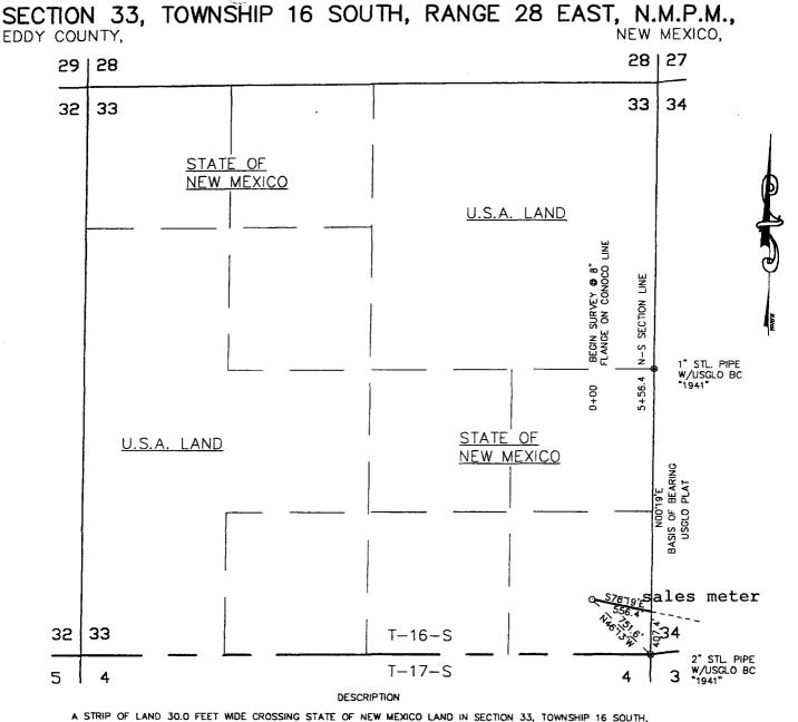
A STRIP OF LAND 30.0 FEET WIDE CROSSING STATE OF NEW MEXICO LAND IN SECTION 33, TOWNSHIP 16 SOUTH, RANGE 28 EAST, N.M.P.M., EDDY COUNTY, NEW MEXICO AND BEING 15.0 FEET LEFT AND RIGHT OF THE FOLLOWING DESCRIBED CENTERLINE SURVEY.
