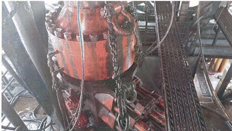
Figure 1: Winch System attached to BOP Stack
