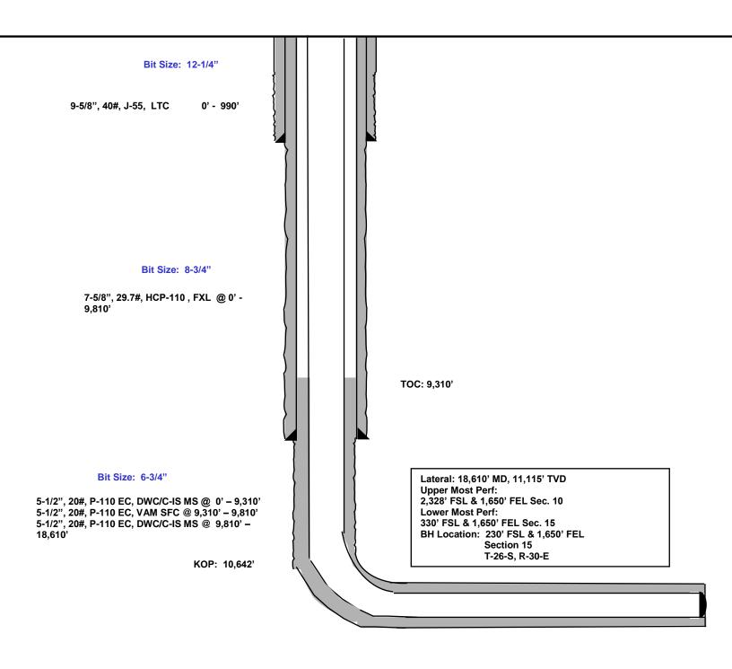
2,460' FSL 1,777' FEL Section 10 T-26-S, R-30-E Proposed Wellbore Design B KB: 3,172' GL: 3,147'
