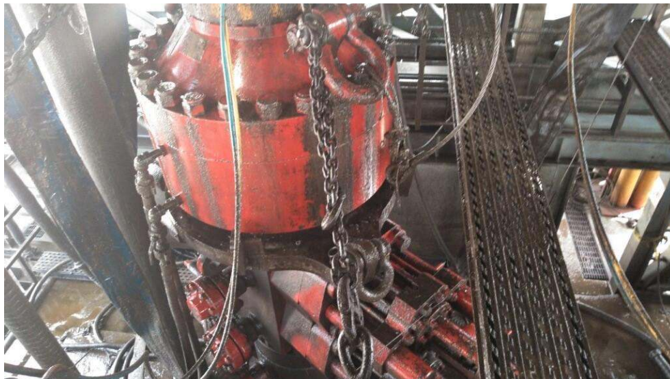
Figure 1: Winch System attached to BOP Stack
