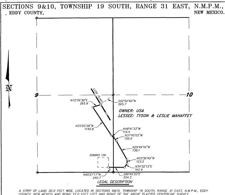
A STRIP OF LAND 30.0 FEET WIDE, LOCATED IN SECTIONS 9&10, TOWNSHIP 19 SOUTH, RANGE 31 EAST, N.M.P.M., EDDY COUNTY, NEW MEXICO AND BEING 15.0 FEET LEFT AND RIGHT OF THE ABOVE PLATTED CENTERLINE SURVEY.
