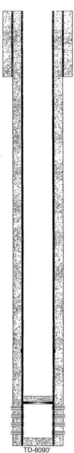
12-1/4" hole @ 1230' 9-5/8" csg @ 1230' w/ 800sx-TOC-Surf-Circ
