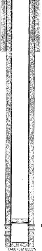
12-1/4" hole @ 1832' 9-5/8" csg @ 1832' w/ 1150sx-TOC-Surf-Circ
