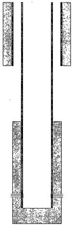
12-1/4" hole @ 959' 8-5/8" csg @ 959' w/ 350sx-TOC-Surf-Circ
