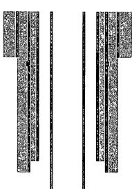
17-1/2" hole @ 416' 13-3/8" csg @ 416' w/ 420sx-TOC-Surf-Circ
