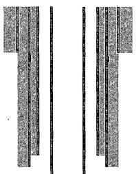
17-1/2" hole @ 416' 13-3/8" csg @ 416' w/ 420sx-TOC-Surf-Circ
