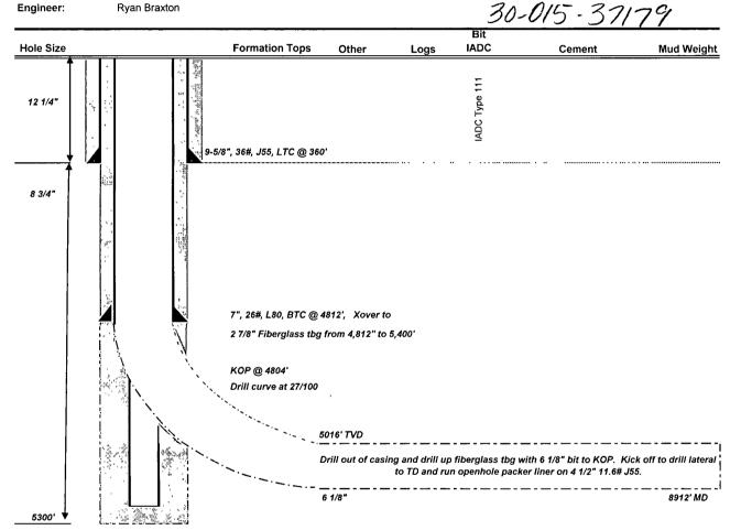
NOTES: Drill to 500'. Run 4812' 7" casing with 2 7/8" fiberglass tubing below to 5400'. Pump cement job to cement fiberglass and casing inplace. With 6 1/8" bit, drill out float collar and drill up fiberglass tubing to KOP. Kickoff and drill lateral to TD. Will run openhole paker liner system on 4 1/2" 11.6# J55 for a 12 stage frac.
