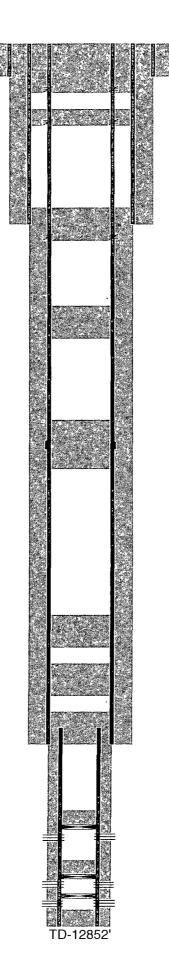
20" hole @ 442' 16" csg @ 442' w/ 510sx-TOC-Surf-Circ
