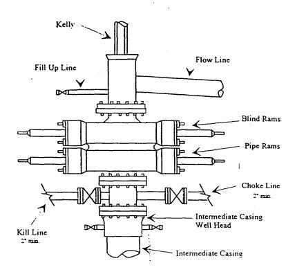
Typical 2,000 psi choke manifold assembly with at least these minimun features
