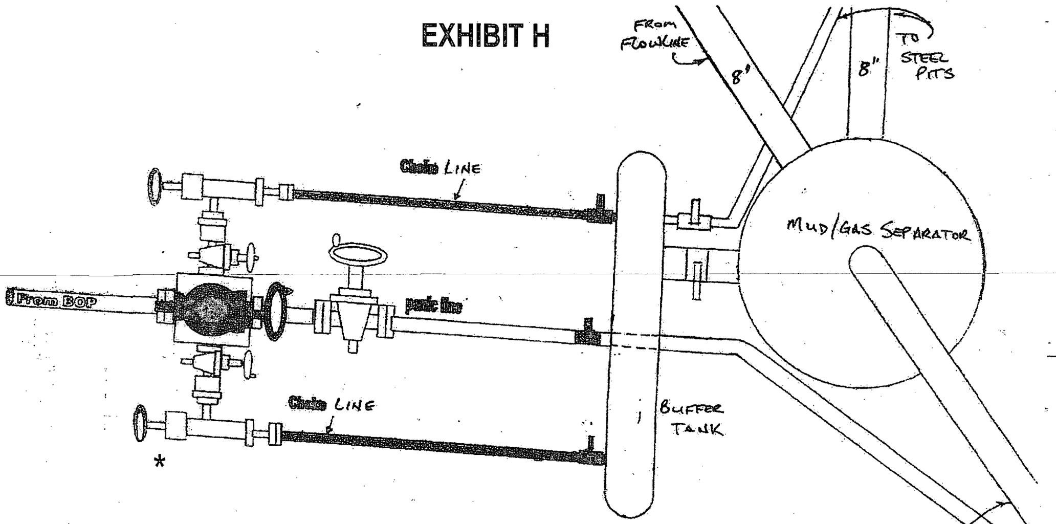
\* Hydraulic Choke Connection Point. Remote control located on rig floor
