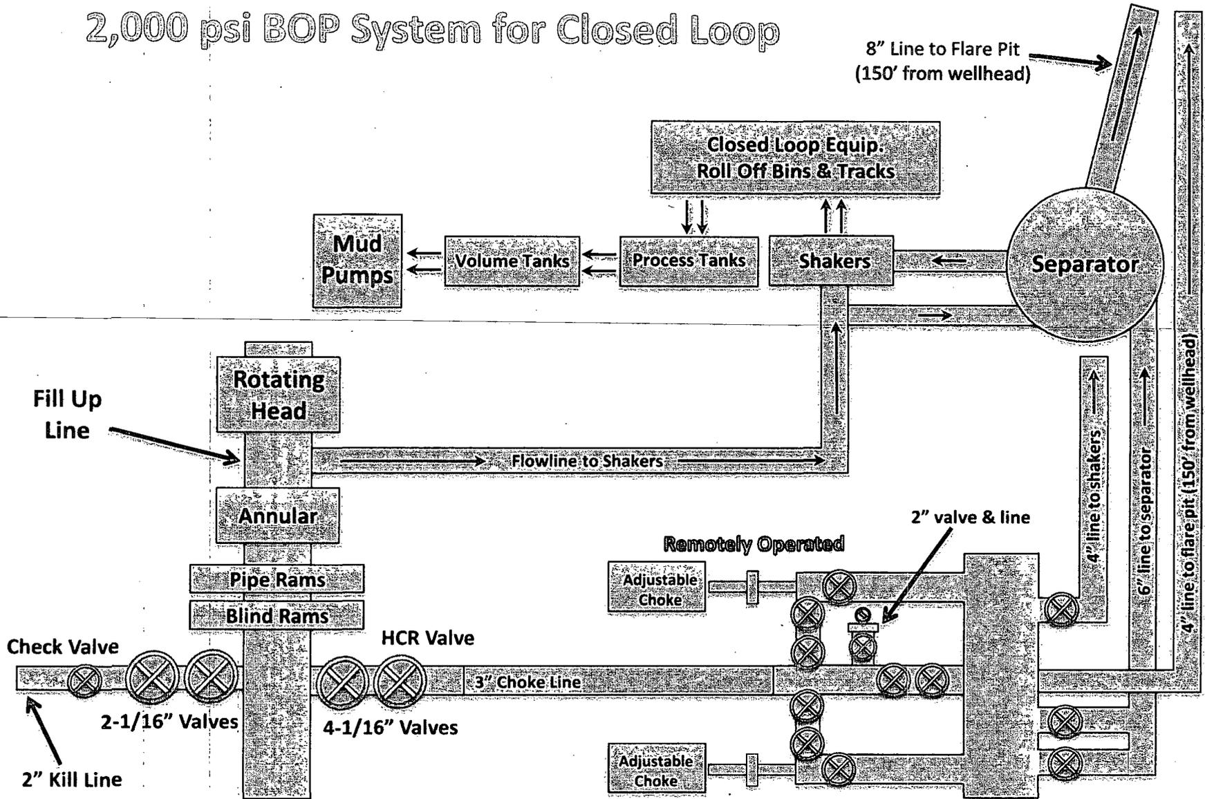
**Note:** All valves & lines on choke manifold are 3" unless otherwise noted. Exact manifold configuration may vary.
