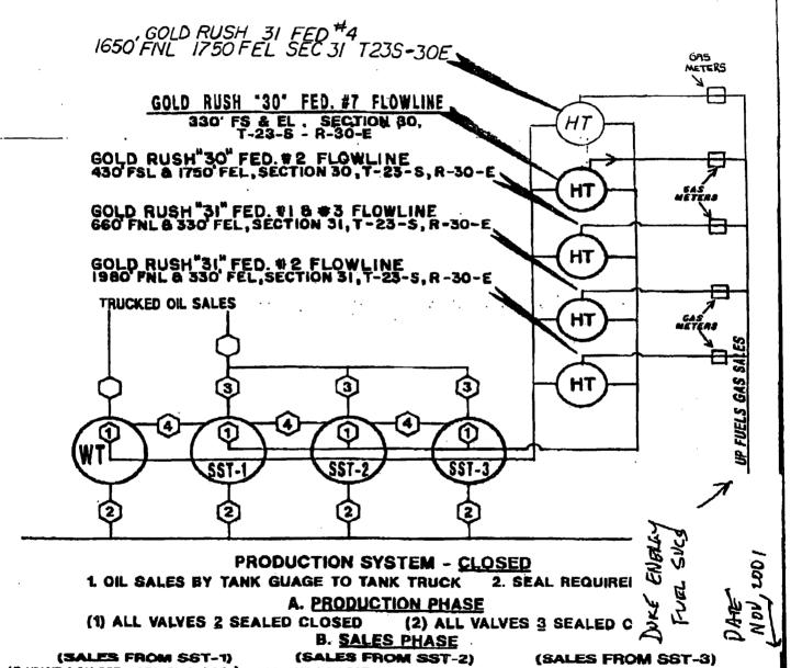
(1) VALVE 1 ON 8ST-1 SEALED CLOSED
