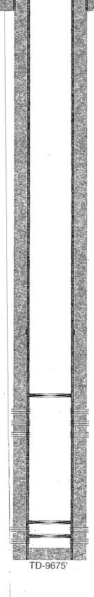
12-1/4" hole @ 1210' 9-5/8" csg @ 1210' w/ 775sx-TOC-Surf-Circ
