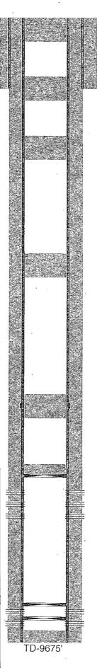
12-1/4" hole @ 1210' 9-5/8" csg @ 1210' w/ 775sx-TOC-Surf-Circ
