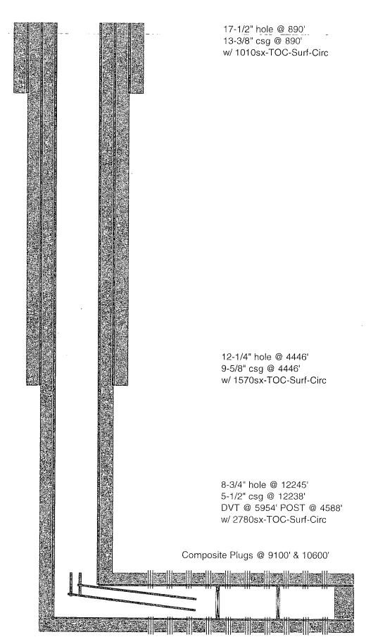
2-3/8" tbg Stuck @ +/- 7340-7600' 2" coil tbg stuck @ +/- 7600-8080'
