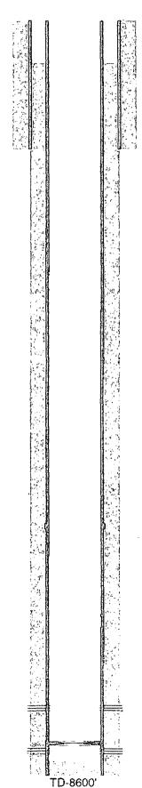
14-3/4" hole @ 1520' 9-5/8" csg @ 1520' w/ 585sx-TOC-Surf-Circ
