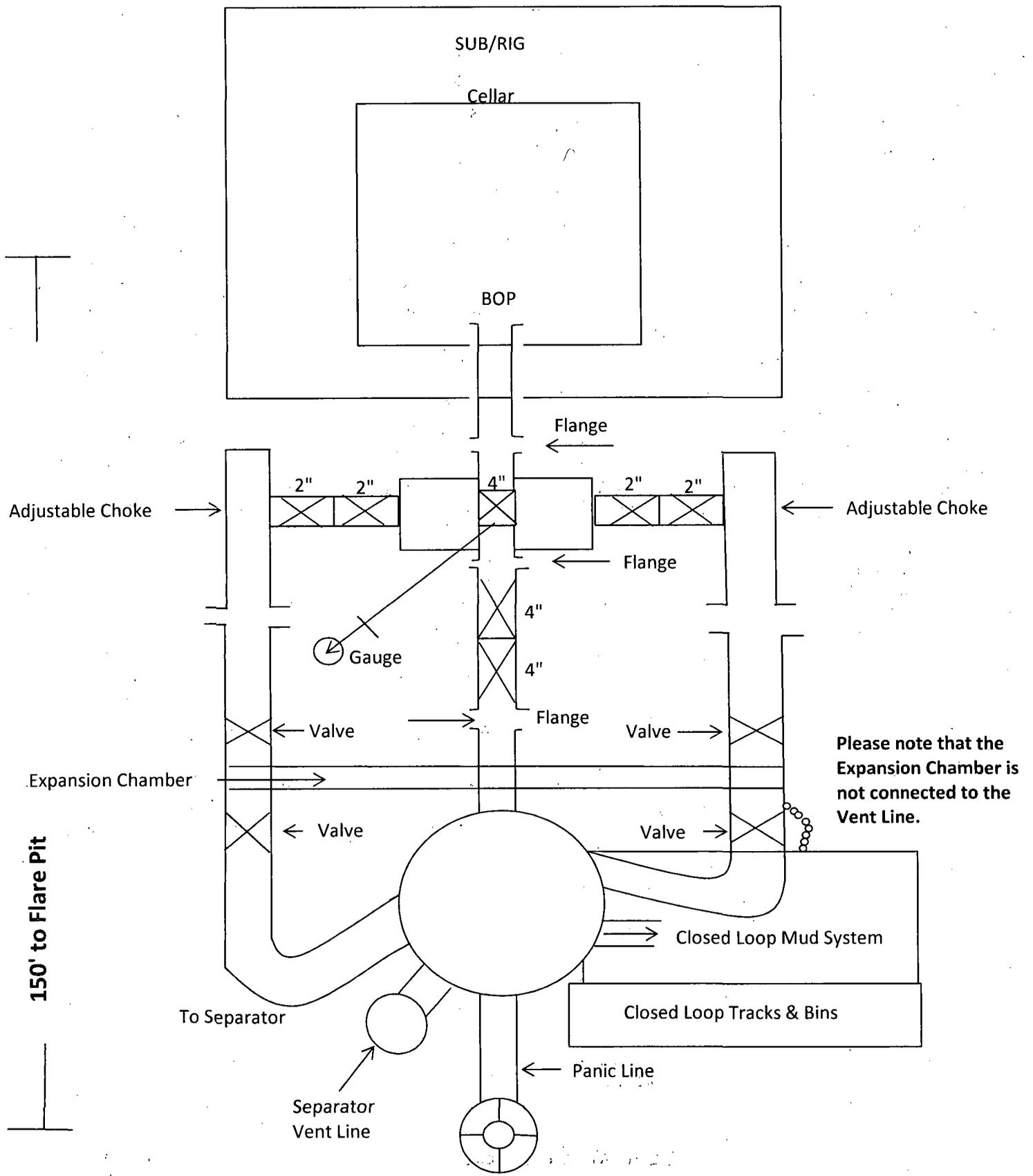
Please note that the Expansion Chamber is not connected to the Vent Line.
