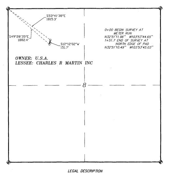
A STRIP OF LAND 30.0 FEET WIDE, LOCATED IN SECTION 8, TOWNSHIP 17 SOUTH, RANGE 31 EAST, N.M.P.M., EDDY COUNTY, NEW MEXICO AND BEING 15.0 FEET LEFT AND RIGHT OF THE ABOVE PLATTED CENTERLINE SURVEY.
