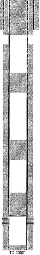
12-1/4" hole @ 351' 8-5/8" csg @ 351' w/ 250sx-TOC-Surf-Circ
