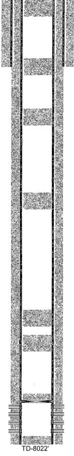
12-1/4" hole @ 1215' 9-5/8" csg @ 1206' w/ 655sx-TOC-Surf-Circ
