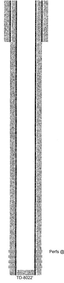
12-1/4" hole @ 1215' 9-5/8" csg @ 1206' w/ 655sx-TOC-Surf-Circ
