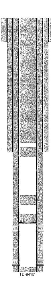
17-1/2" hole @ 850' 13-3/8" csg @ 850' w/ 900sx-TOC-Surf-Circ
