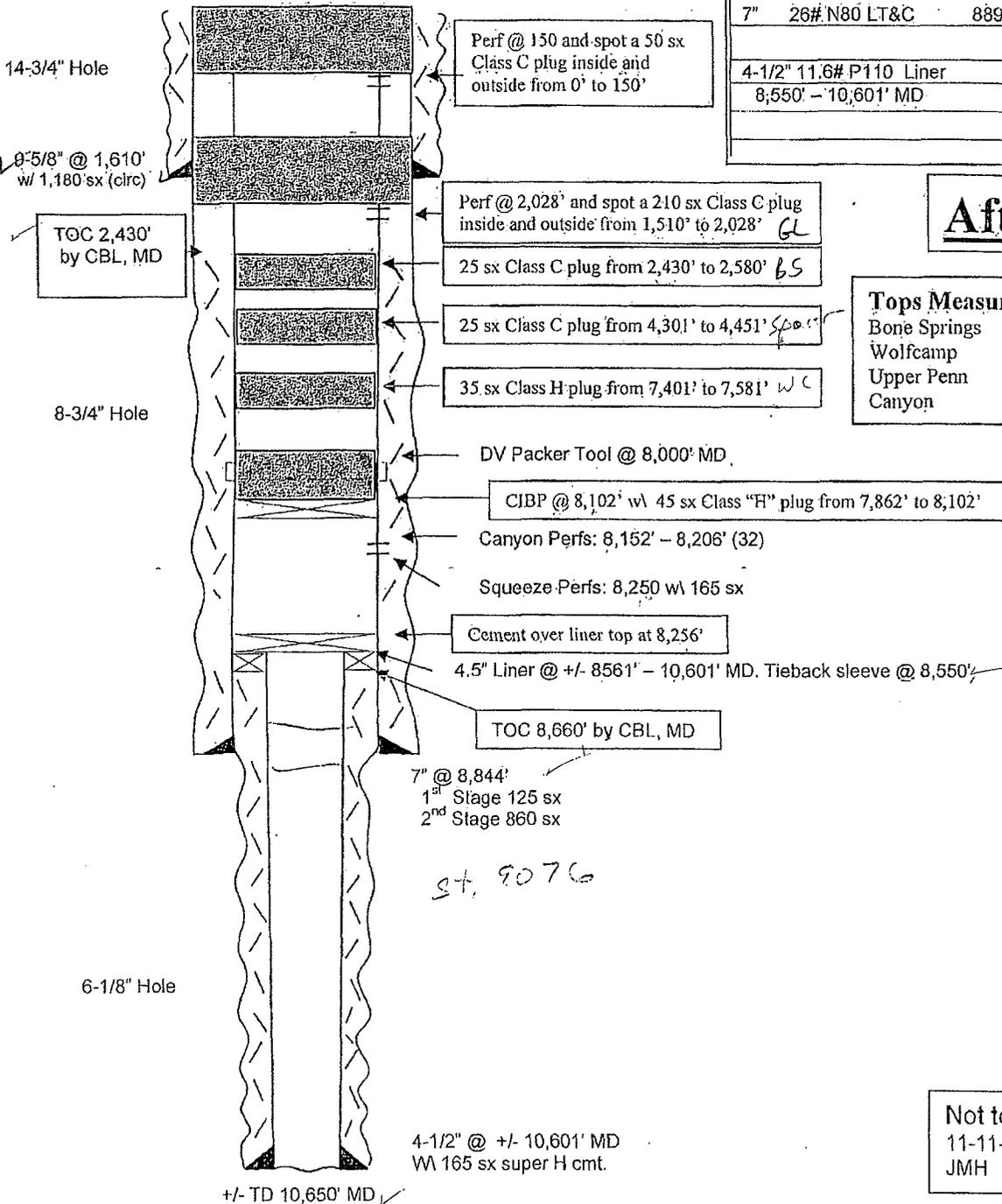
Perf @ 150 and spot a 50 sx Class C plug inside and outside from 0' to 150'
