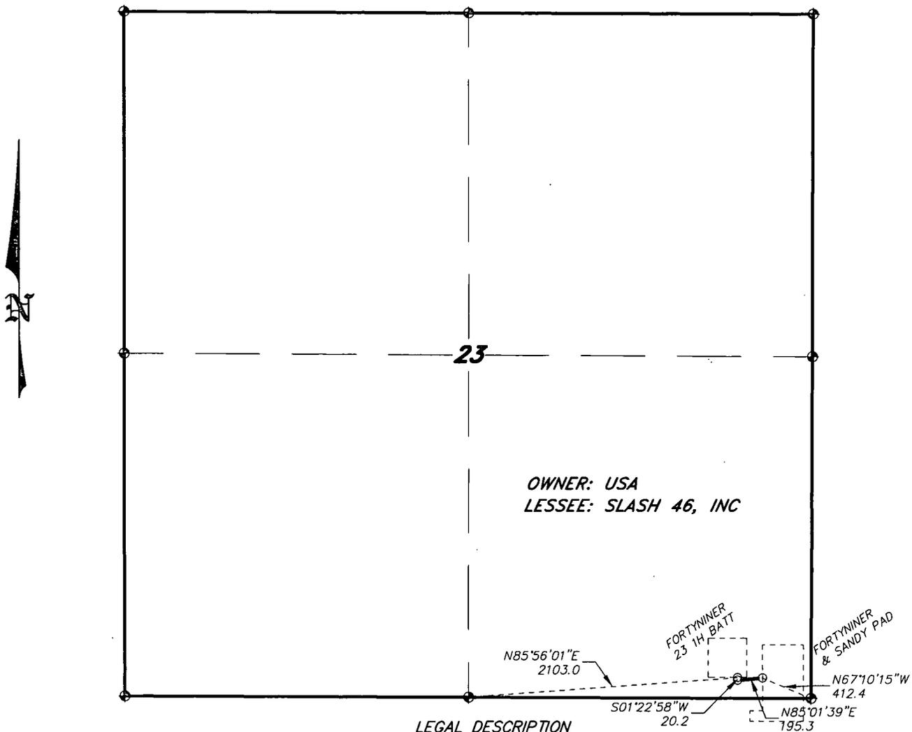
A STRIP OF LAND 30.0 FEET WIDE, LOCATED IN SECTION 23, TOWNSHIP 23 SOUTH, RANGE 30 EAST, N.M.P.M., EDDY COUNTY, NEW MEXICO AND BEING 15.0 FEET LEFT AND RIGHT OF THE ABOVE PLATTED CENTERLINE SURVEY.
