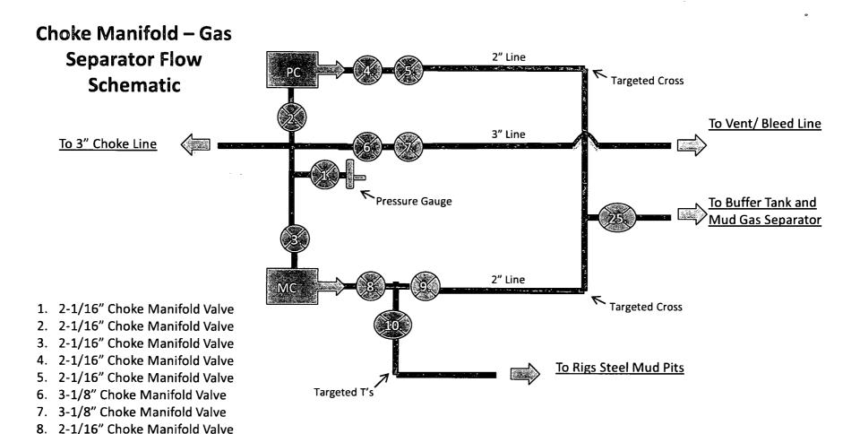
\* All T's in the choke manifold and coming off of the choke manifold will be targeted.
