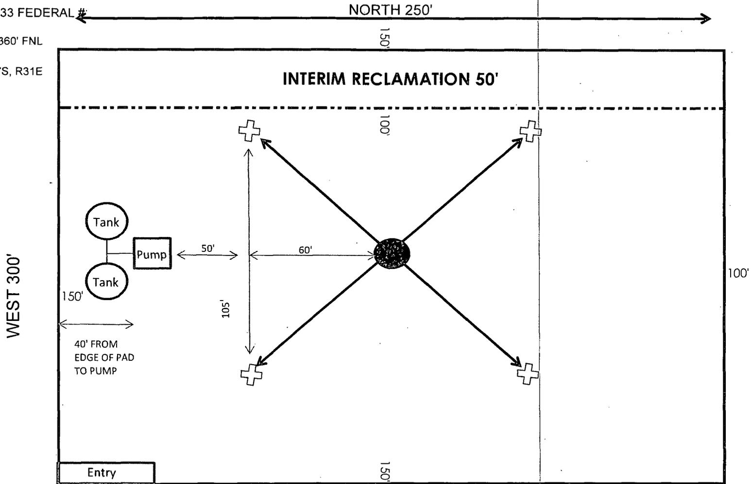
✚ ANCHOR 75' FROM WELLHEAD TO ANCHORS
