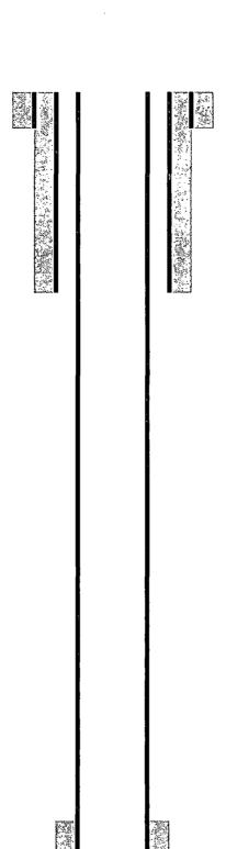
17-1/2" hole @ 200' 13-3/8" csg @ 200' w/ 250sx-TOC-Surf-Circ
