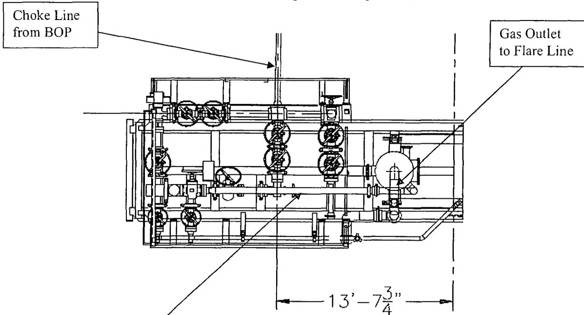
Choke Manifold – Gas Separator (Side View)
