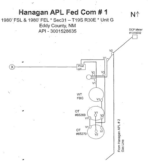
V1= Valve Closed V2= Valve Opened
