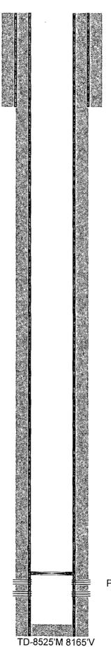
17-1/2" hole @ 1414' 13-3/8" csg @ 1400' w/ 2000sx-TOC-Surf-Circ
