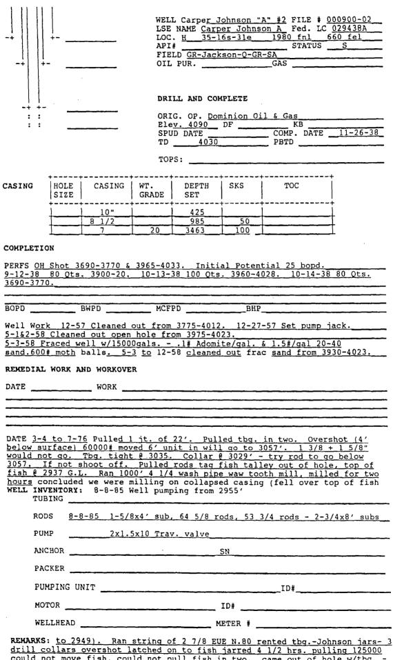
could not move fish, could not pull fish in two. came out of hole w/tbg. - jars. Ran tbg rods hung well back on production 30 foot off fish
