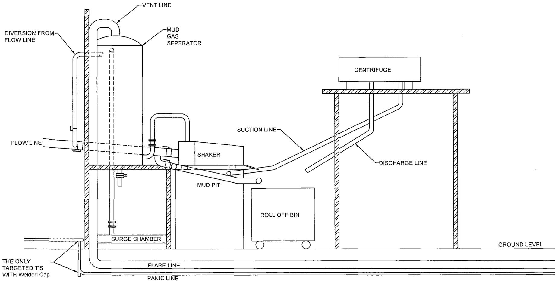
The flare discharge must be 100' from wellhead for non H2S wells and 150' from wellhead for wells expected to encounter H2S.
