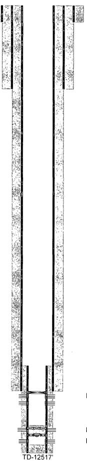
17-1/2" hole @ 400' 13-3/8" csg @ 399' w/ 420sx-TOC-Surf-Circ
