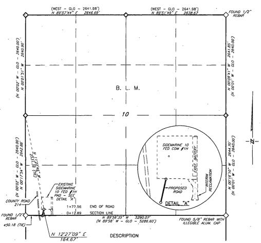
A strip of land being 30 feet in width, being 164.67 feet or 9.980 rods in length situated in Section 10, Township 17 South, Range 29 East, N. M. P. M., Eddy County, New Mexico, being 15 feet left and 15 feet right of the following described survey of a centerline across the land of the B. L. M.:
