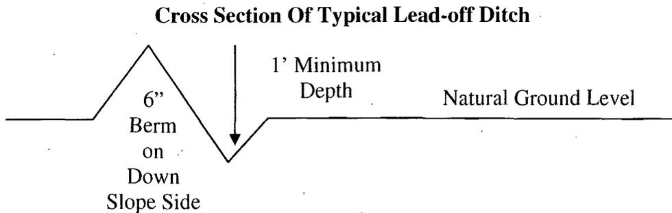
All lead-off ditches shall be graded to drain water with a 1 percent minimum to 3 percent maximum ditch slope. The spacing interval are variable for lead-off ditches and shall be determined according to the formula for spacing intervals of lead-off ditches, but may be amended depending upon existing soil types and centerline road slope (in %);
