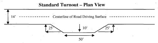
Drainage control systems shall be constructed on the entire length of road (e.g. ditches, sidehill, out-sloping and in-sloping, lead-off ditches, culvert installation, and low water crossings). A typical lead-off ditch has a minimum depth of 1 foot below and a berm of 6 inches above natural ground level. The berm shall be on the down-slope side of the lead-off ditch.
