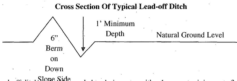
All lead-off ditches shall be graded to drain water with a 1 percent minimum to 3 percent maximum ditch slope. The spacing interval are variable for lead-off ditches and shall be
