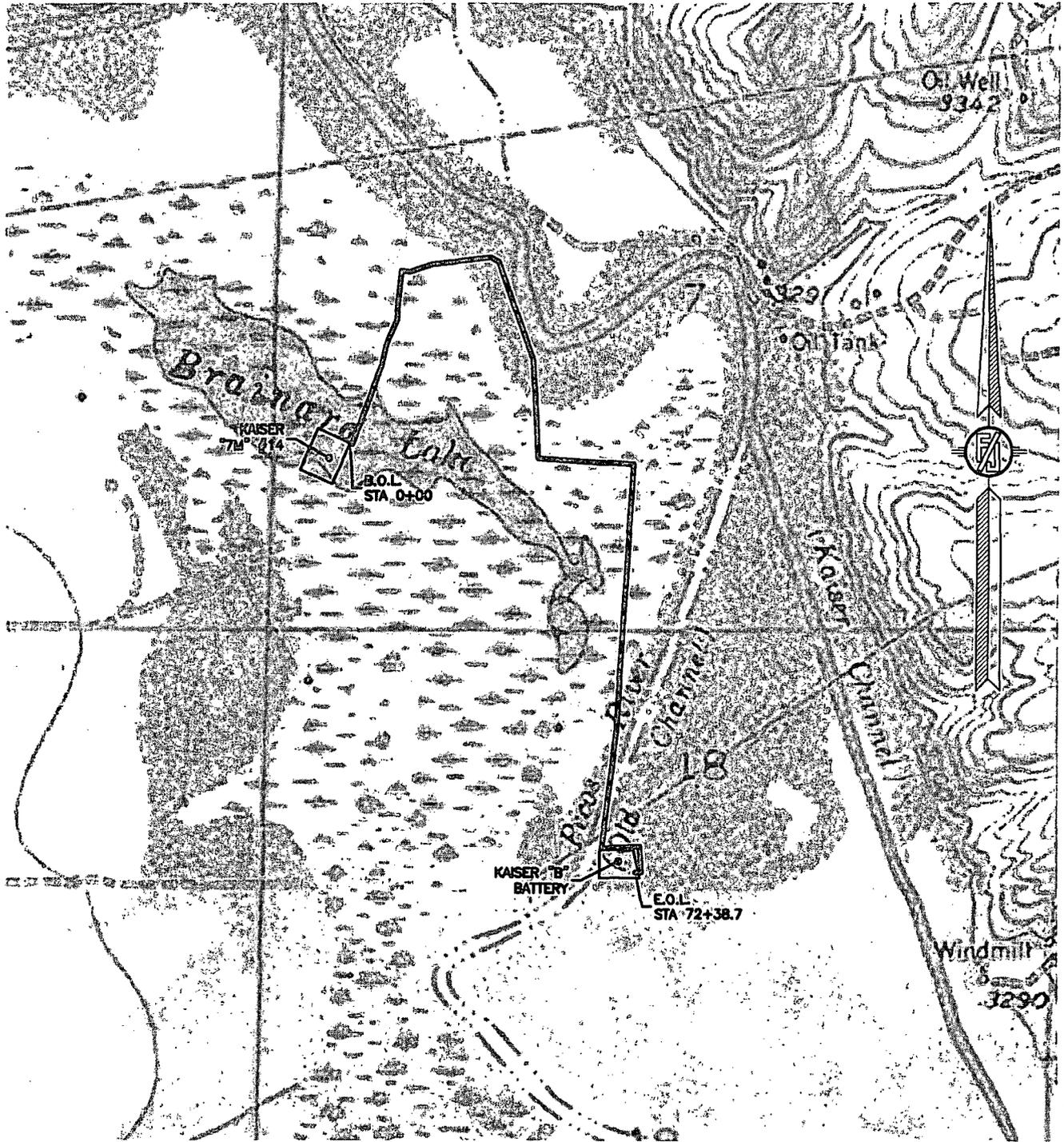
R-0-W FOR TWO 3" SDR 7 POLY SURFACE LINES (ONE GAS AND ONE PRODUCTION)
