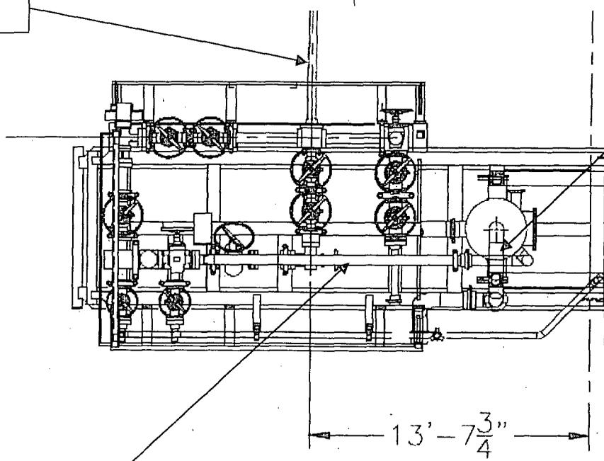
Choke Manifold – Gas Separator (Side View)
