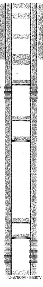
12-1/4" hole @ 1811' 9-5/8" csg @ 1811' w/ 1950sx-TOC-Surf-1"-Circ
