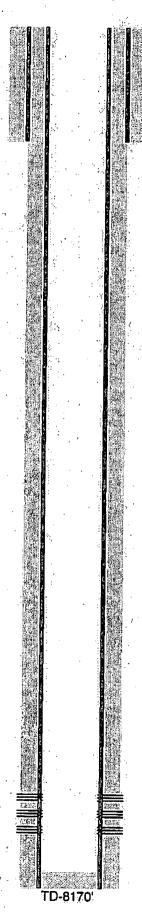
12-1/4" hole @ 1201' 9-5/8" csg @ 1201' w/ 700sx-TOC-Surf-Circ
