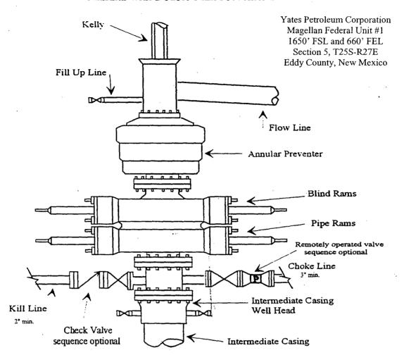
Typical 5,000 psi choke manifold assembly with at least these minimun features
