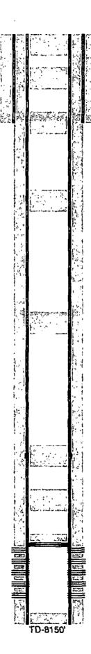
12-1/4" hole @ 1230' 9-5/8" csg @ 1230' w/ 740sx-TOC-Surf-Circ
