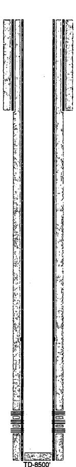
12-1/4" hole @ 1800' 9-5/8" csg @ 1798' w/ 900sx-TOC-Surf-Circ
