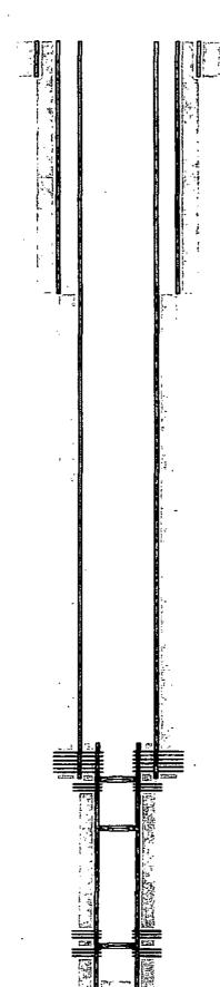
17-1/2" hole @ 430' 13-3/8" csg @ 430' w/ 475sx-TOC-Surf-Circ
