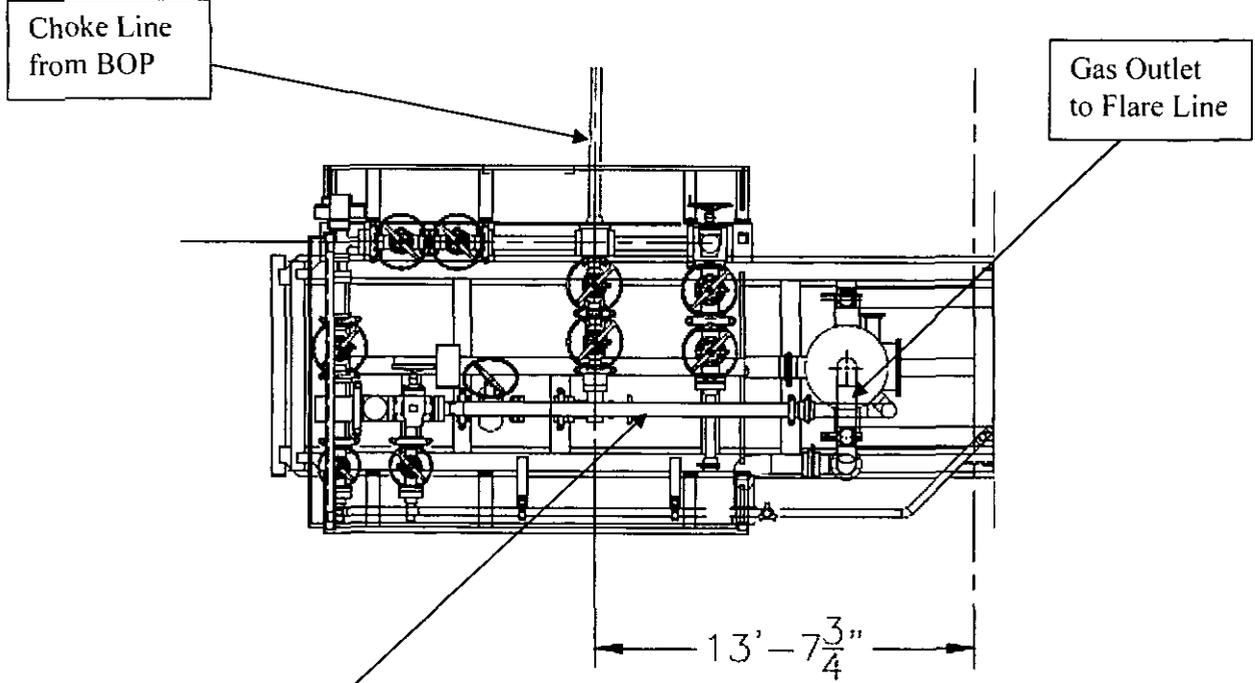
**Choke Manifold – Gas Separator (Side View)**
